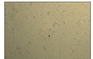
Oil sample taken 110 days AFTER installation of CJC™ Oil Filter ISO 16/15/11
