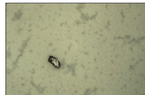
Oil sample taken BEFORE installation of CJC™ Oil Filter ISO 20/18/15
