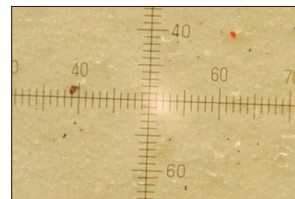
Oil sample membranes BEFORE CJC™ Pressure Kit
