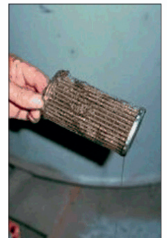
A used inline filter
