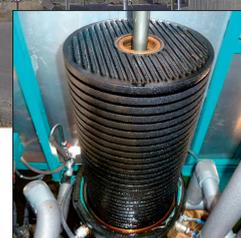
CJC™ Varnish Removal Insert, VRi after 30 days of operation
