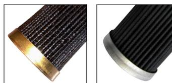
Varnish coated in-line filter of IGV servo valve hydraulics, before and after filtration with CJC™ VRU
