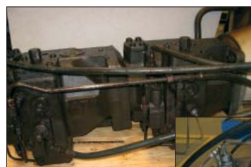
The submerged pump for the hydraulic press BEFORE CJC™ Filtration
