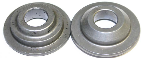
Hardened parts: on the left with unfiltered , on the right with filtered quenching bath
