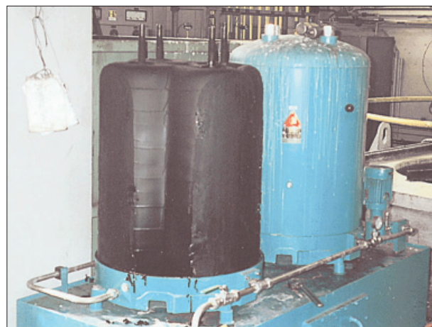
Changing the first set of inserts in the HDU 2 x 427/81 MZ-EPQTVY on the 40,000 litre system
