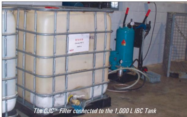
*The CJC™ Filter connected to the 1,000 L IBC Tank*
