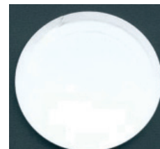
Membrane AFTER CJC™ Filtration
