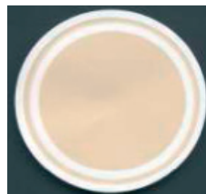
Membrane BEFORE CJC™ Filtration
