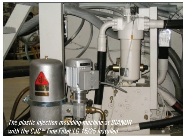
The plastic injection moulding machine at BIANOR with the CJC™ Fine Filter LG 15/25 installed
