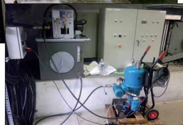
CJC™ Filter Separator PTU 27/27 Mobile
