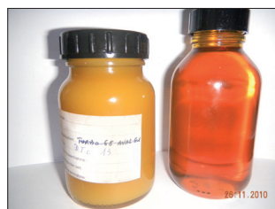
Oil samples before and after one day with CJC™ Filtration
