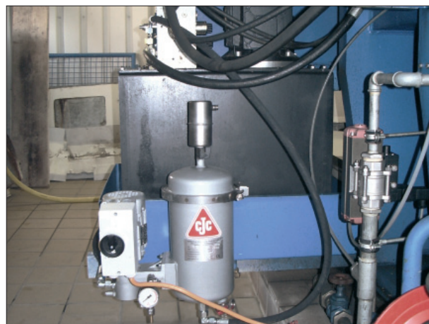
CJC™ Fine Filter HDU15/25 P installed at hydraulic tank of a chamber filter-press
