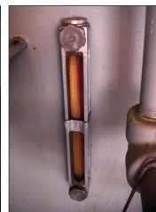
Sight glass, AFTER CJC™ Oil Filtration
