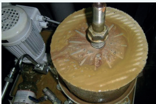
Dirty CJC™ Filter Insert, saturated with highly emulsified EAL oil. After filtration, the stern tube oil is now free of water.
