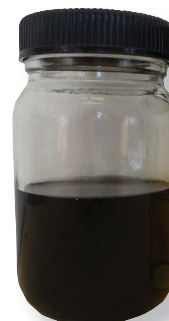
Transformer 1 without CJC™ Filter
