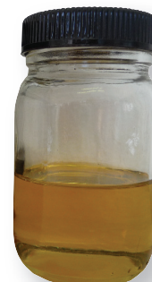
Transformer 8 with CJC™ Filter
