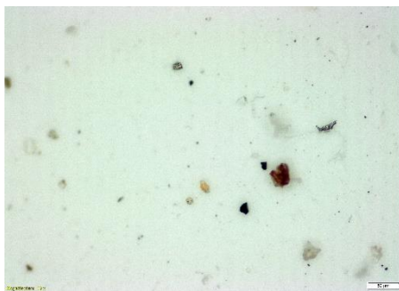
Membrane, hydraulic oil under microscope, particle visualisation
